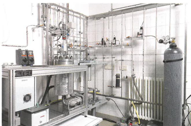
FIG. 2. Pilot plant in Leipzig, Germany, with autoclaves for under-critical and overcritical conditions.
