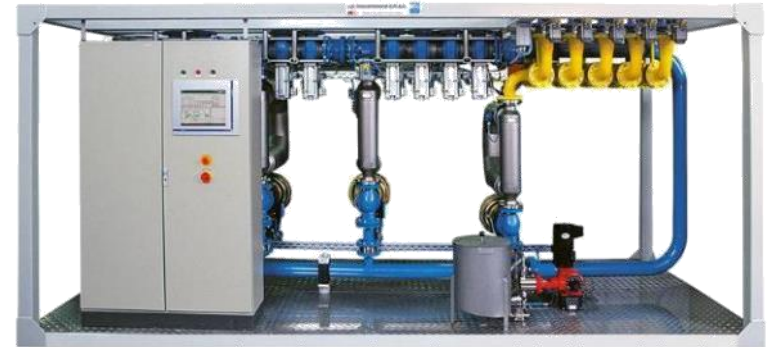
Skid-mounted Simultaneous Metering Blender
