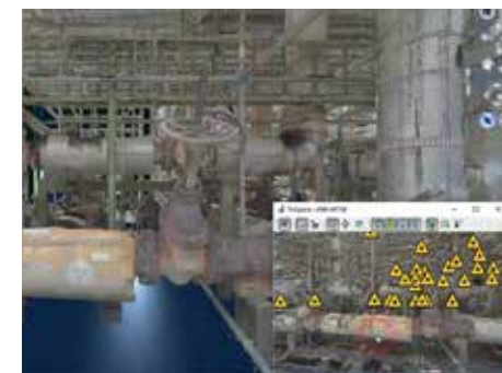
Point cloud of a plant unit, the little section shows the scan points in yellow
