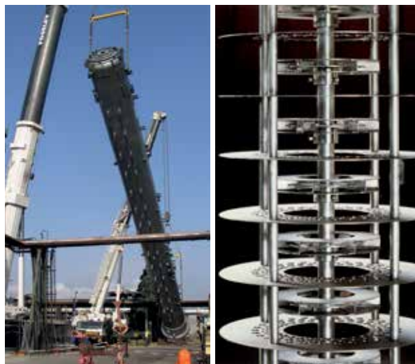
Fig. 3: Extraction column with agitated internals by Sulzer (left), highly efficient agitated column internals by Sulzer (right)
