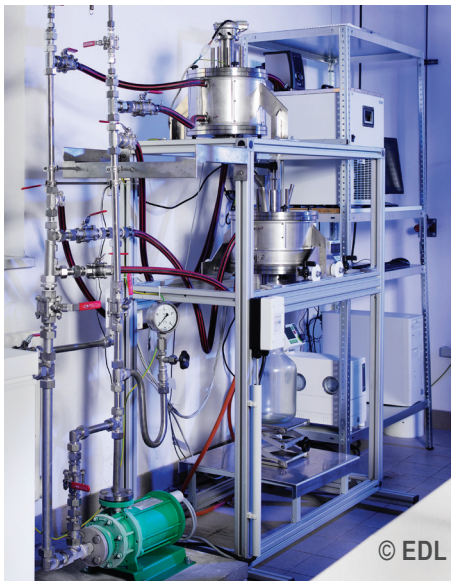
EDL-Pilot plant for the solvent process
