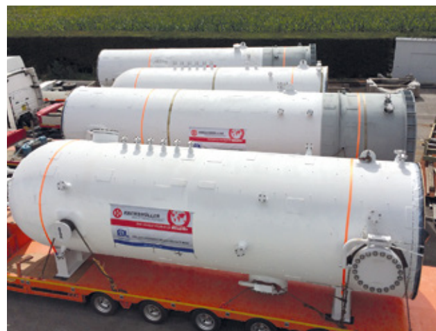
Fig. 4: OAO Naftan, Novopolozk, Belarus: Engineering and delivery of two extractors for conversion of PDA plant
