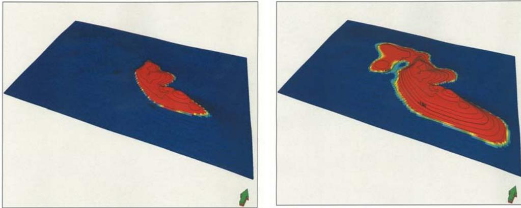
Fig. 11 - Identification of gas losses – gas saturation after simulating the correct storage operation in comparison with gas saturation after simulating the historic, real and incorrect storage operation (red = gas, blue = water)
