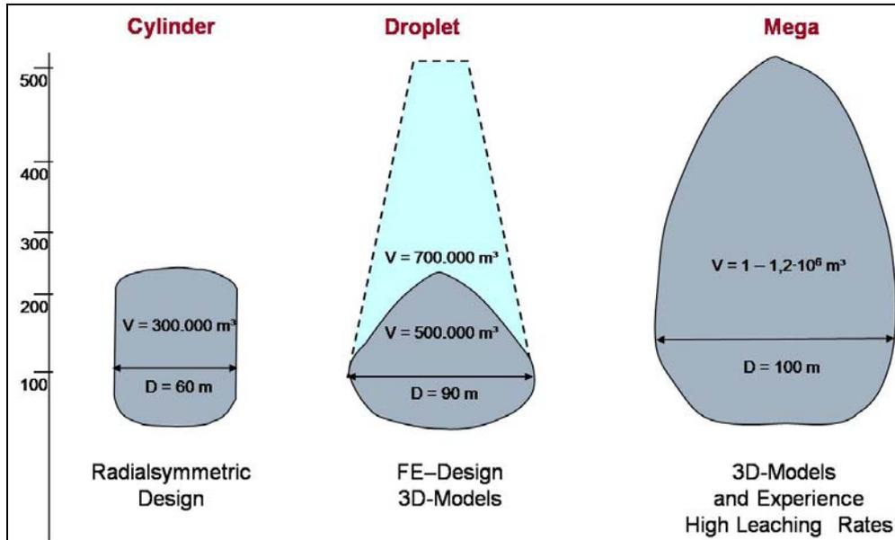
Fig. 4 - Examples of different shapes and sizes of salt caverns
