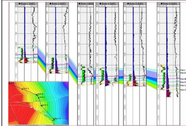
Fig. 5 - Cross section with geophysical well LOGs
