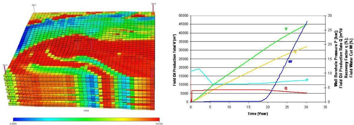
Fig. 9 - 3D-reservoir model and diagram with production curves of a production for water flooding
